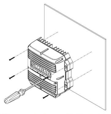
→ Note: Where possible, mount the processor in a way that the LEDs indicators may be viewed if required for diagnostic purposes.
